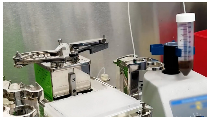
Third-party shaker combines with the Mantis to ensure homogeneity of beads
