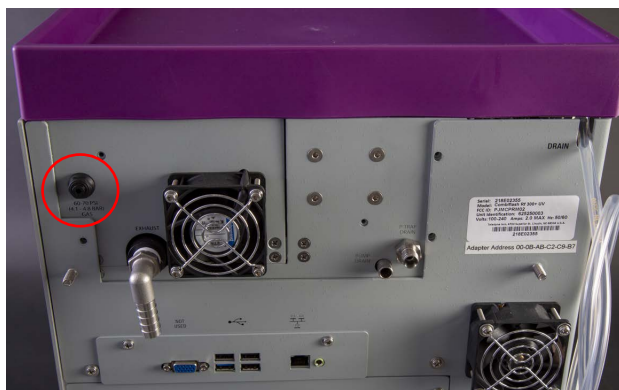
Figure 2-4 Location of ELSD gas port (Nitrogen input line circled)
