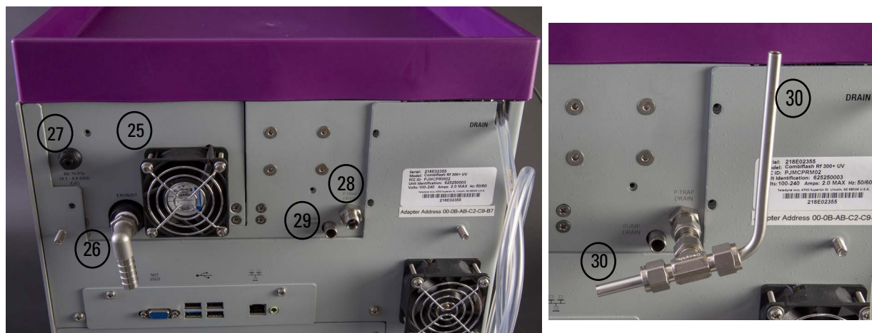
Figure 1-8 CombiFlash NextGen ELSD (back) and P-Trap Drain Vent Assembly
