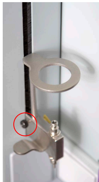
Figure 2-12 Location of the side hole to secure the SLCC ring support
